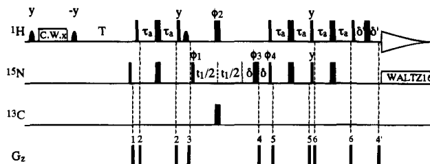
Figure 12. Pulse scheme for the measurement of HN T_1 values. All narrow (wide) pulses have a flip angle of 90^\circ ( 180^\circ ). Unless otherwise indicated the phase of all of the pulses is x . The shaped ^1\text{H} pulses are either 2 ms 90^\circ rectangular pulses or 2 ms pulses having the SEDUCE-1 44 profile and are selective for water. A 7 kHz C.W. pulse (along the x axis) is applied for 60 ms between the first two shaped pulses to completely randomize ^1\text{H} magnetization from the protein so that at the start of the recovery period, T , the protein magnetization has the initial condition M_z = 0 , while for water the magnetization is close to the equilibrium value. ^{15}\text{N} decoupling during acquisition is achieved using a 1 kHz WALTZ 45 field, while ^{15}\text{N} pulses are applied using a 5.3 kHz field. The carbon 180^\circ pulse is applied using an 18 kHz field centered at 117 ppm, approximately midway between the ^{13}\text{C}^\alpha and the ^{13}\text{C}' resonances. The delays used are \tau_a = 2.4 ms, \delta = 1.4 ms, \delta' = 0.5 ms. The phase cycling employed is \phi_1 = x ; \phi_2 = x, -x ; \phi_3 = 2(x), 2(y), 2(-x), 2(-y) ; \phi_4 = x ; \text{rec} = 2(x), 2(-x) . For each value of t_1 , N- and P-type coherences are obtained by recording two data sets whereby the sign of the gradient g_4 is inverted and 180^\circ added to the phase of \phi_4 for the second data set. Data sets obtained for positive and negative g_4 values are stored in separate memory locations and pure absorptive line shapes in the ^{15}\text{N} dimension generated by adding and subtracting the N- and P-type data sets, storing the new data sets separately, and applying a 90^\circ zero-order phase correction in the acquisition dimension to one of the new data sets. 25 The phase of \phi_1 and the phase of the receiver are incremented by 180^\circ for each increment of t_1 . 51 The durations and strengths of the gradients (rectangular) are g_1 = (1.0 ms, 8 G/cm), g_2 = (0.5 ms, 8 G/cm), g_3 = (1.5 ms, 15 G/cm), g_4 = (1.25 ms, 30 G/cm), g_4' = (0.125 ms, 27.8 G/cm), g_5 = g_6 = (0.4 ms, 4 G/cm).
